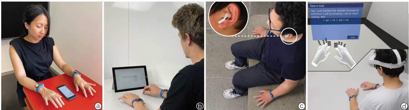
Figure 1: TapType is a portable, wireless text entry system that brings touch typing to everyday surfaces. TapType’s two wristbands sense vibrations arising from finger taps, from which our Bayesian classifier estimates finger probabilities. Our text decoder then estimates input character sequences by fusing these predictions with the priors of an n -gram language model given a key-finger mapping. TapType is suitable for several applications, including text entry (a) on a phone or (b) on a tablet using the surrounding surface for increased typing convenience, (c) in conjunction with audio feedback only in mobile scenarios, or (d) in situated Mixed Reality to complement typing with passive haptic feedback.
