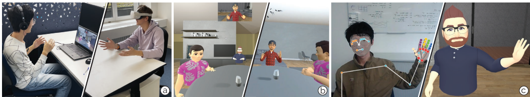
Fig. 1. ViGather is a teleconferencing system that integrates users of traditional screen devices (e.g., PCs, laptops, tablets) and Mixed Reality users wearing headsets into a joint experience. ViGather represents all users through embodied and animated avatars that reflect the verbal and non-verbal interaction between users in a shared virtual environment. (a) A laptop user emphasizes his statements through hand gestures while videoconferencing with a user of an immersive system. (b) ViGather represents both users as avatars in the same virtual environment, rendering each participant’s experience from a first-person perspective on their respective display. (c) To animate avatars’ non-verbal communication cues, our system tracks body language and gaze direction using the sensors inside the headsets for Mixed Reality users, while it processes the front-facing camera feed to extract the same behavioral cues on traditional screen devices.
