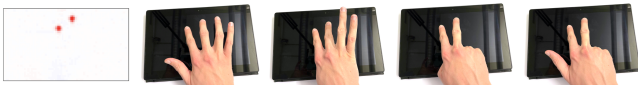
Figure 7: The same capacitive image (left) can result from different hand poses due to variations in orientation of fingers that are not touching the screen. Here, only index and middle fingers are touching the screen.
